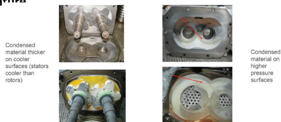
Figure 4. Condensation occurs locally where temperatures are low or pressures high.
